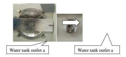
'Water tank outlet a' is used for draining. Please plug a specialized connector in the 'outlet a'. Push the little slice on the top of the connector to pull out the draining
