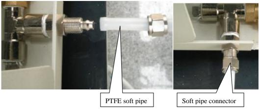
Before drainage, a PTFE soft pipe (attached accessories) should be connected to the outlet. Please use specialized rotate tool.
