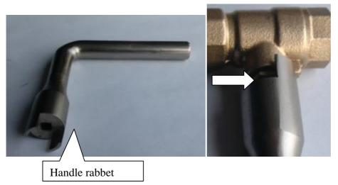
Plug ledge of the ball valve into the handle rabbet and twist  $90^\circ$  to drain water. Twist the handle  $90^\circ$  reversely after drainage.
